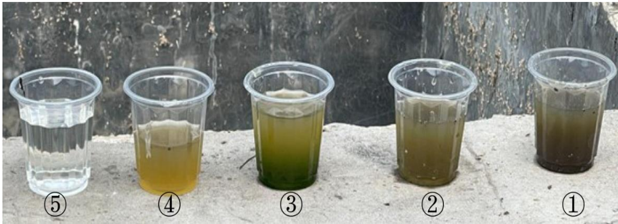
Fig. 5.7 Progressive clarification of aquaculture wastewater through microbial treatment and duckweed polishing. The photograph displays samples (5)–(1) from left to right, whereas treatment proceeds from (1) to (5). Sample (1) is untreated aquaculture wastewater; samples (2)–(4) are the effluents after the first, second, and third microbial reactors, respectively; and sample (5) is the final effluent after the additional duckweed-polishing stage.
